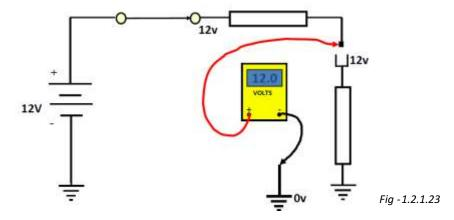
Voltage potential is the voltage that is present at a point in a circuit when the load or ground has been disconnected.
