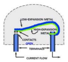
Fig. 2.1.7 Circuit Protection
