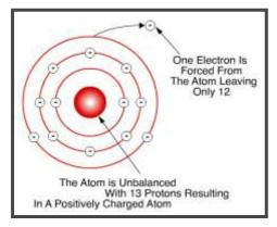
When something upsets this balance, then some of the **Electrons** become out of the orbits. (**Free Electrons**) this unbalanced condition can be caused by rubbing (heat), passing a wire through a Magnetic Field or putting two chemicals together (as in a Dry Cell Battery).
