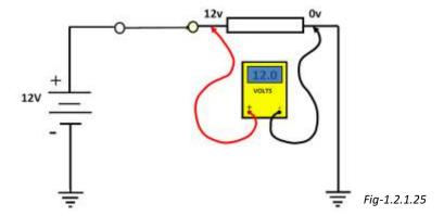
**Voltage drop** is the difference of voltage values between the meter leads. When the leads are Connected to each side of a light bulb (load), the meter measures voltage into the bulb. The other lead measures the voltage out. The meter reads the voltage difference on the display. In a series circuit with one light bulb, the total source voltage will drop across the bulb.
