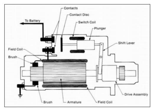
Fig. 1.3.7 Starter Motor
