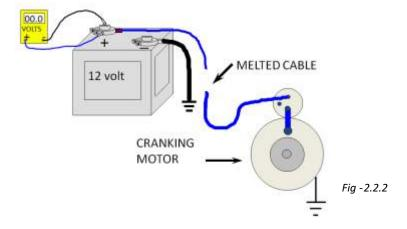
The cable could not handle the amperage because it was too small so it melted.
