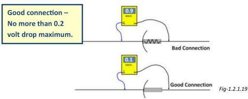
A good connection is no more than 0.2 volt drop maximum. We will show you what a bad connection will look like in the shop. A connection can be a switch, relay contacts, circuit breaker, etc.
