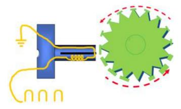
Fig. 2.1.6 Magnetic pick up Unit
