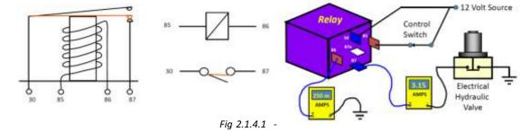
Do we have to pass voltage? No. We could pass ground.
