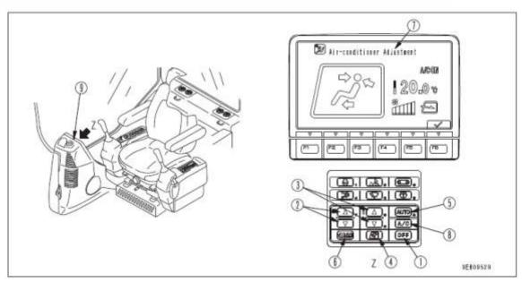
Fig. 1.3.3 Air Conditioner Control Panel
