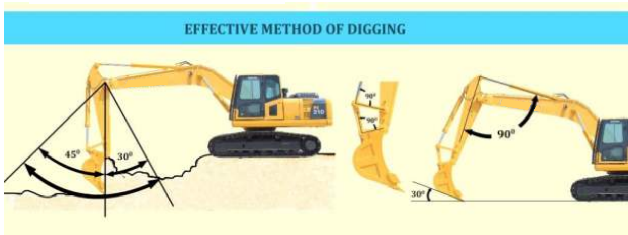
Fig 3.2.1 (c) Effective Digging Angles
