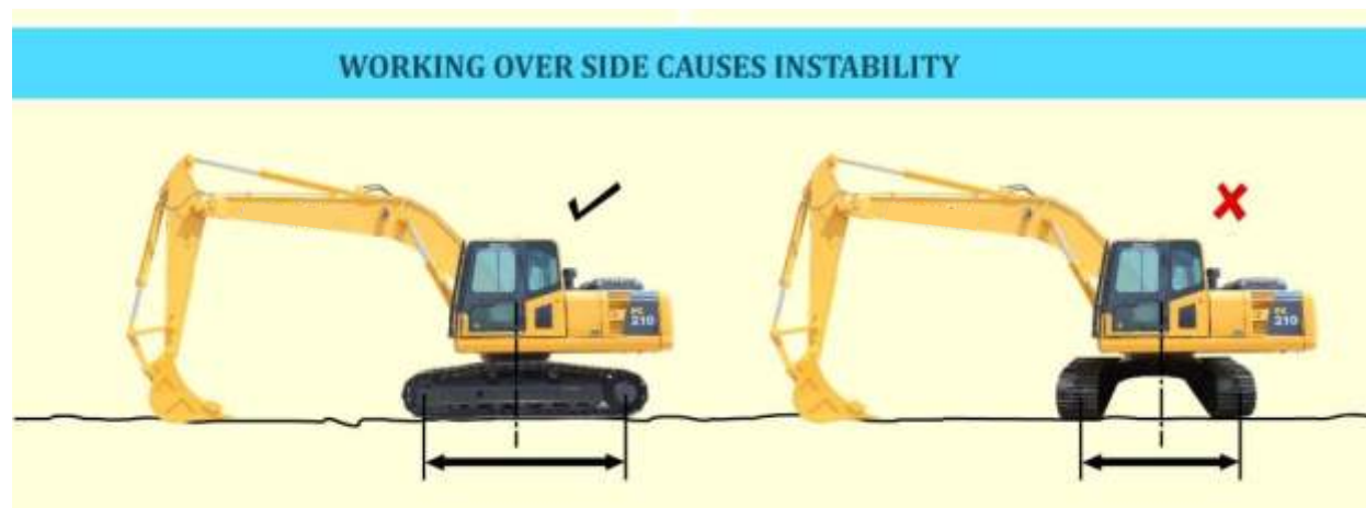
Fig 3.2.1 (b) Excavator working over side
