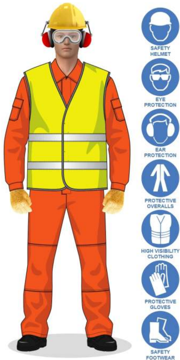
Fig 5.2.1 (c) Personal Protective Equipment for Worksite
